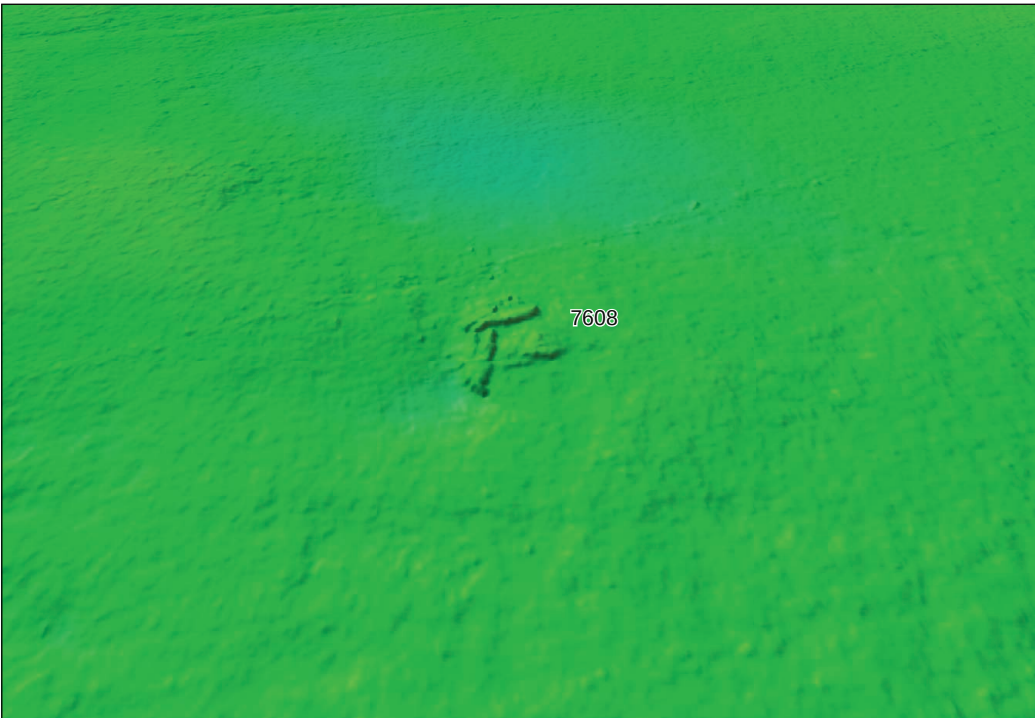
Anomaly 7608 (UKHO_91237), MBES grid image, x1 vertical exaggeration, looking north
