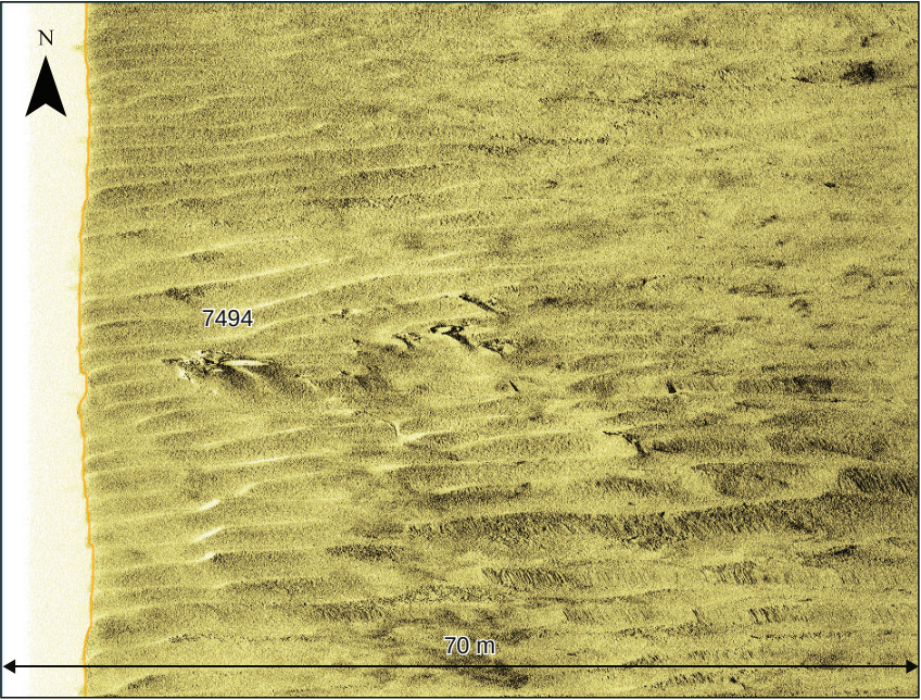
Sidescan sonar waterfall image of wreck 7494 , 70 m range per channel
